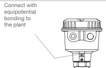
Version with seperate housing must be grounded additionally at the vibrating fork.
