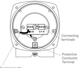
Ground-Terminal on the electronic module is connected internally to the housing (not all versions)
