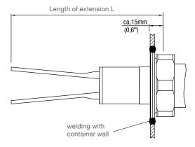
Dimension of flush welding socket (for optional on site manufacturing):
